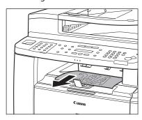
When outputting LGL size paper, lift the paper stopper to prevent the paper from falling off the output tray.
